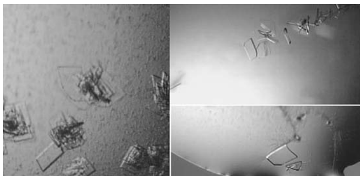
Figure 1 Monoclonic crystals of the glycogen synthase of A. tumefaciens , which are plates of dimensions 0.1 \times 0.1 \times 0.03 mm.
